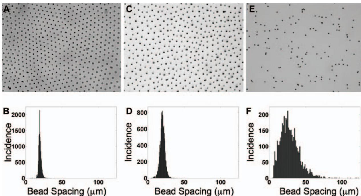
**FIG. 5.** Phase-contrast micrographs of bead patterns (A, C, E) and histograms of the inter-bead spacing distribution (B, D, F) within samples. Highly ordered micro-bead arrays were created with magnetic guidance when applied to beads present in phosphate-buffered saline (A, B) or fibrinogen solution (C, D) with the external magnet system, whereas random bead distributions were formed in fibrinogen solution (E, F) in the absence of an applied magnetic field.
