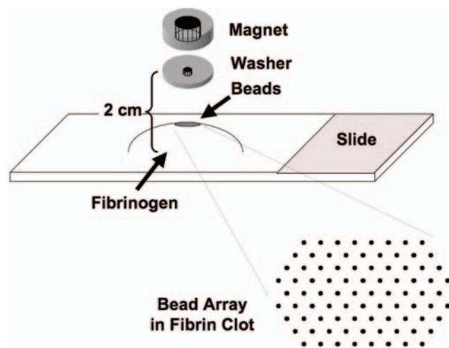
**FIG. 1.** Schematic diagram of the magnetic bead array guidance system. Color images available online at [www.liebertpub.com/ten](http://www.liebertpub.com/ten).
