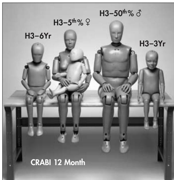
FIGURE 2 The Hybrid III (H3) frontal-impact family. Courtesy of First Technology Safety Systems.
