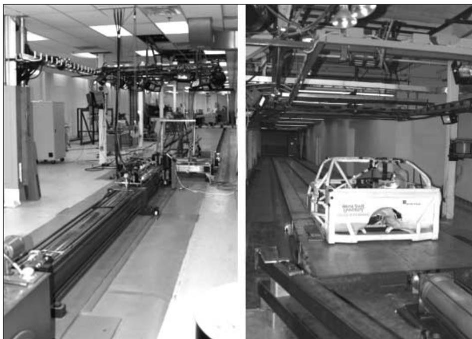
FIGURE 1 1a. HYGE acceleration sled.
