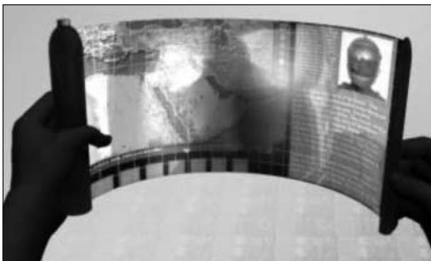
FIGURE 2 Wireless flexible display for use by the soldier on the battlefield. Source: Eric Forsythe and David Morton, Army Research Laboratory.
