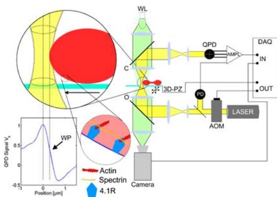
*Fig 4: Set-up for measuring membrane fluctuations of liposomes. T. Betz, unpublished results*
