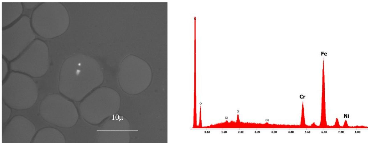
Fig. 1 - Nanoparticles in a red cell and EDS spectrum.
